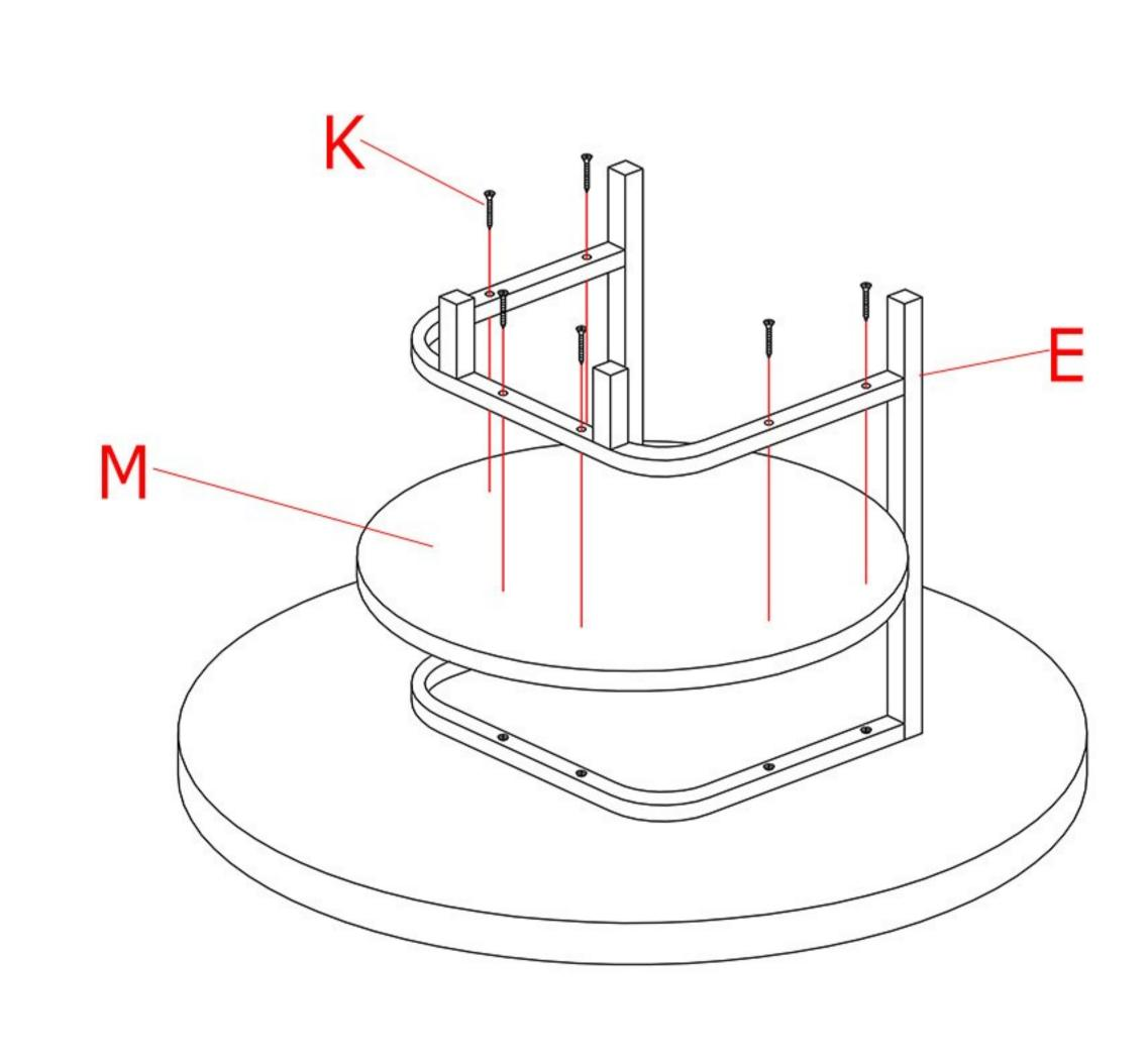
4. Center the back of the small round board (M) to the arch frame (E) and fix it with long self-tapping screws (K) as shown.
