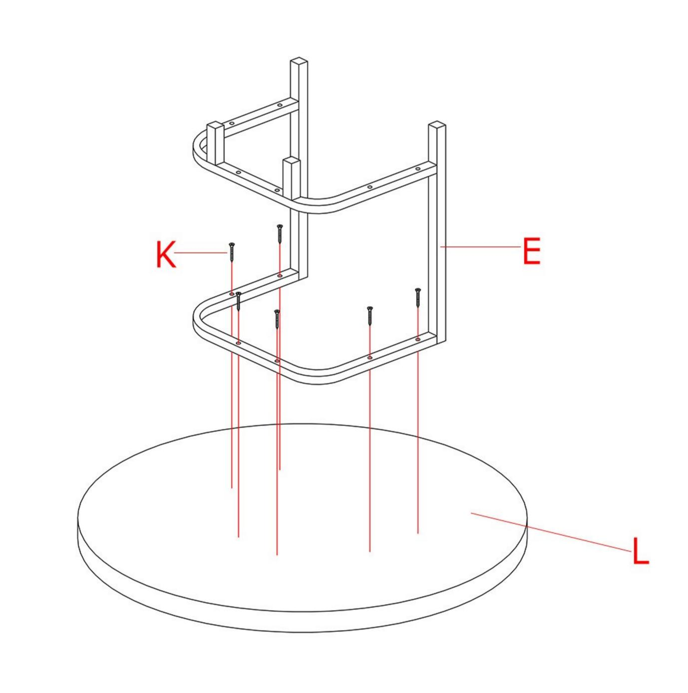
3. Place the big round board (L) upside down on the floor and the arch frame (E) on the the big round board. Center the board and fix the board to the frame by driving the long self-tapping screws (K) through the holes on the frame into the board.
