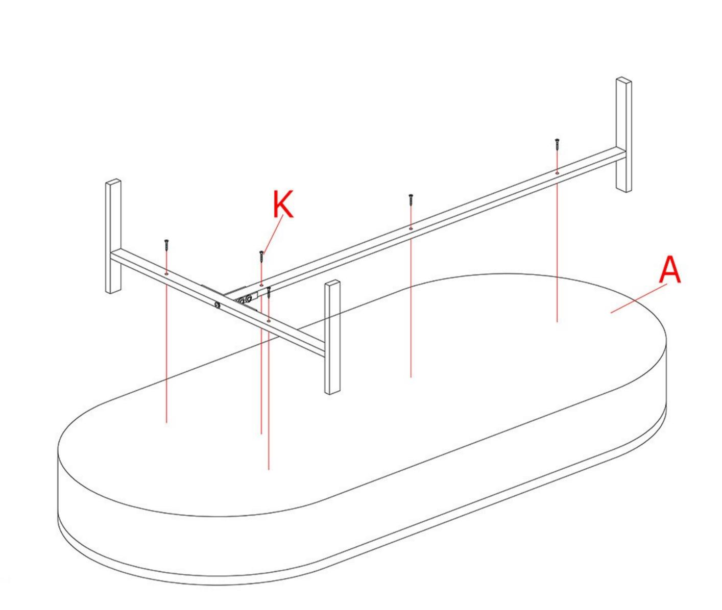
1. Align one end of T-shape frame (B) to H-shape frame (C) at the central hole and fix them by screwing on a medium screw (G) and gasket (J) through the hole of H-shape frame into the T-shape frame. Align bent metal straps (D) with the T-shape frame and H-shape frame hole by hole and fix them with short screws (F) and gaskets vertically through the holes of bent metal straps to H-shape and long screws (H) and screw nuts (I) vertically through the holes of bent metal straps to the T-shape.
